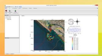
It can be used either as a real-time basis to predict the sedimentation or as a scenario model to analyse the possible impact of sediments due to constructions of piles, jetties and ports
