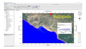
POLSOFT provides rapid predictions of the pollutant dispersion in any meteorological and hydrological conditions. It includes user friendly graphical interface for entering both wind and hydrological data
